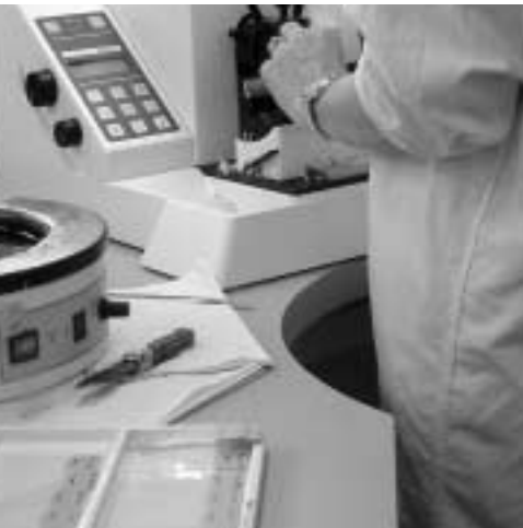
The histology workstation cut-out reduces reaches and allows closer access to equipment
