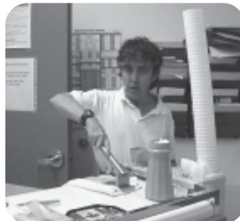
Awkward postures and forceful exertions are required to push down on the lever arm of a standard pill crusher.
