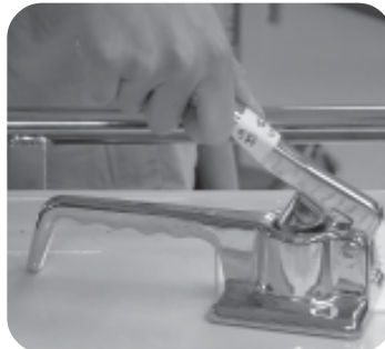
A standard pill crusher consists of a metal head attached to a lever arm.
