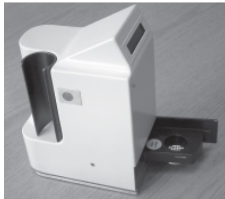
Left: The automated pill crusher (prototype #5). Pills are placed between two medication cups and placed on the plastic base, which is then rotated closed to seal the crushing chamber.
